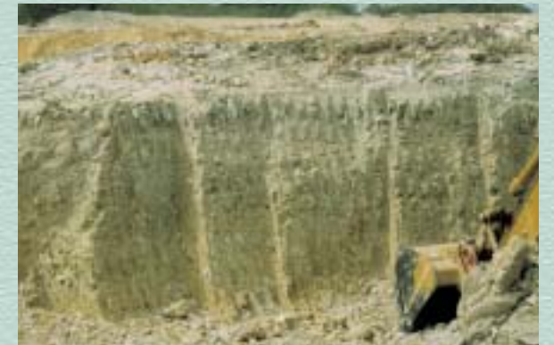
Ball clay being selectively extracted from the Creekmoor Clay, Doreys Pit.
